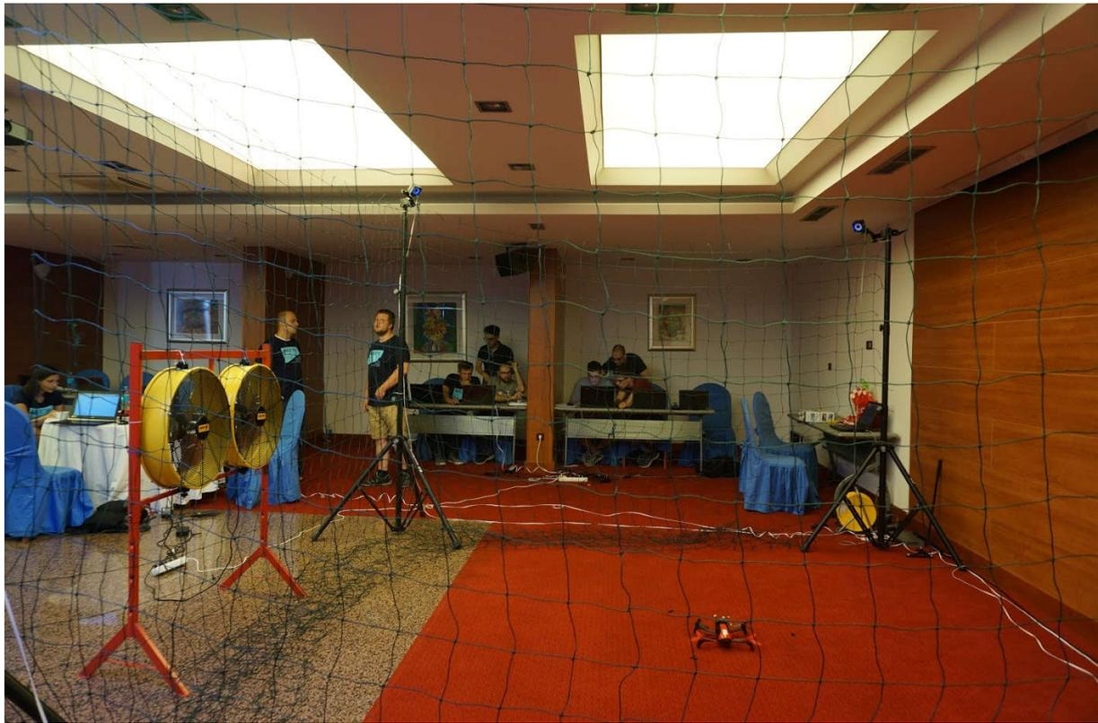
Figure 5 - Aerial robotics control and perception challenge mockup wind farm environment
